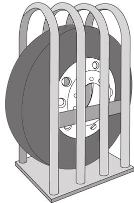
Place the tyre in an inflation safety cage and inflate the tyre to the required pressure value.
